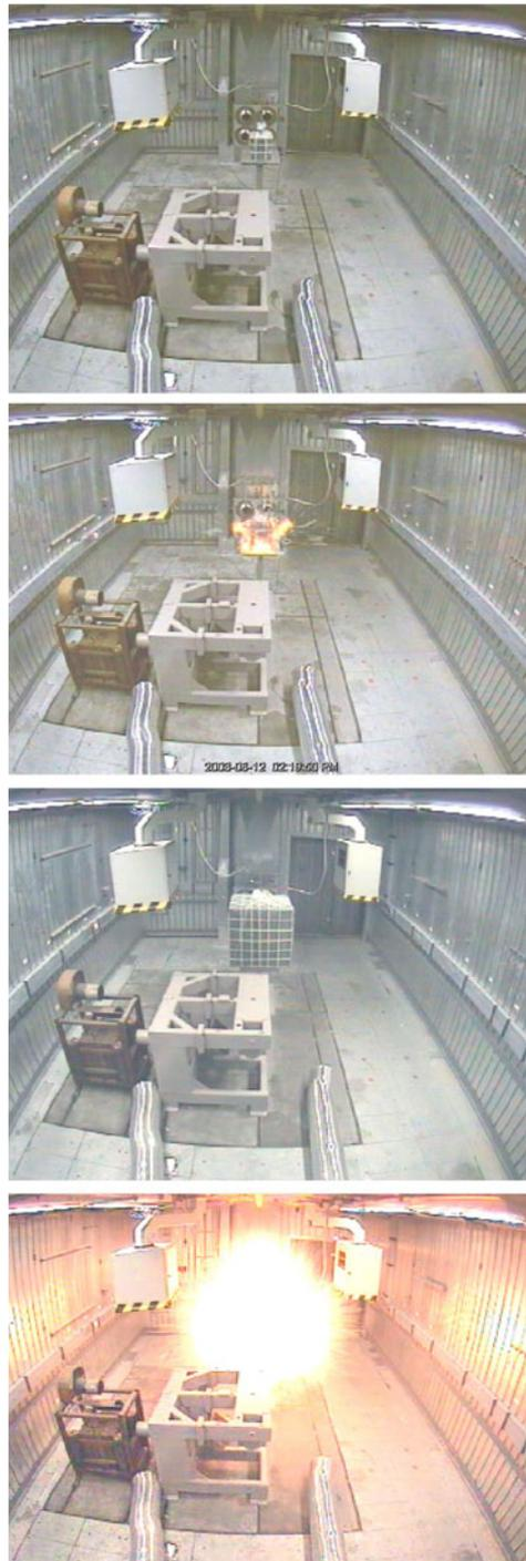
**Figure 12.** Hydrogen deflagration and detonation tests within structural enclosure (Singh *et al* 2003, 2004a, b).
