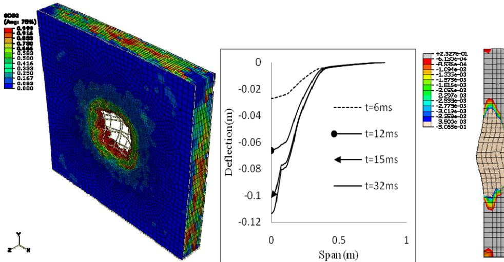
Punching and Flexure failure modes in RC slab
