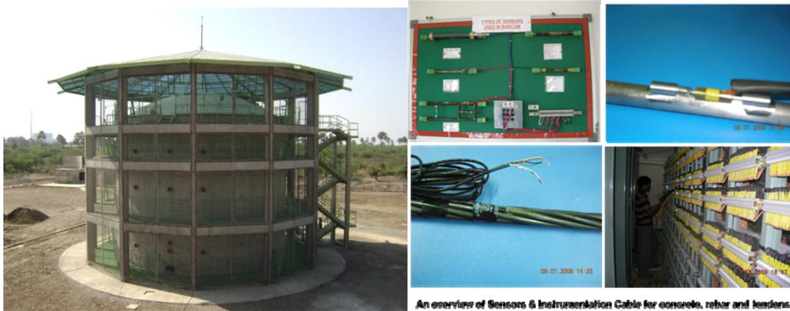
**BARC Containment (BARCOM) Test-Model (Design Pressure Pd 0.1413 MPa)
