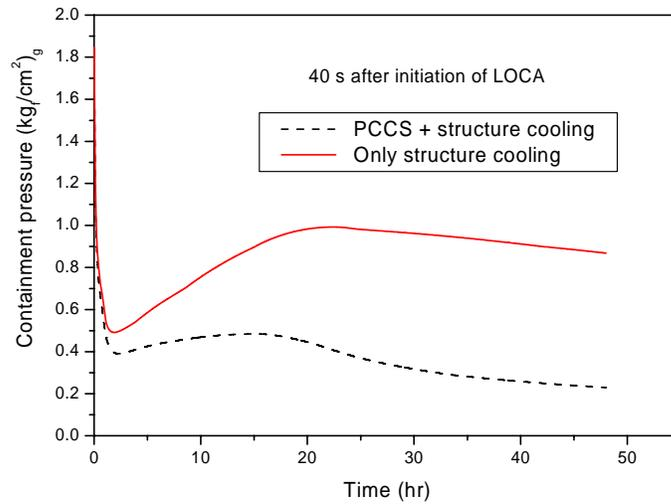
**Containment pressure transients considering PCCS and concrete cooling**
