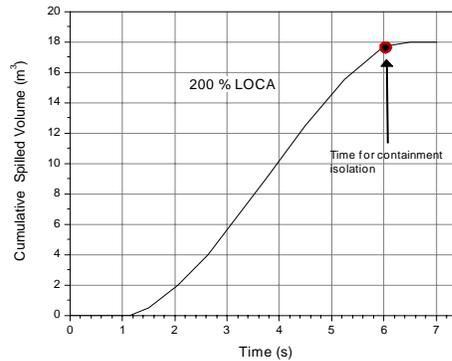
Cumulative Water Spillage in U duct
