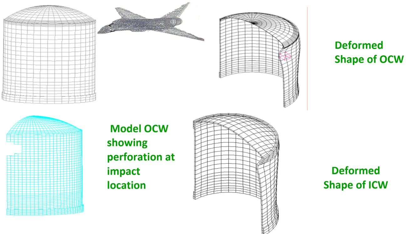
**540 MWe PHWR Accidental Aircraft Impact Simulation for ICW and OCW
