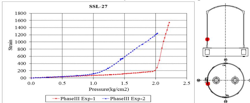
Response during Over-Pressure Test in BARCOM near MAL at SSL-27
