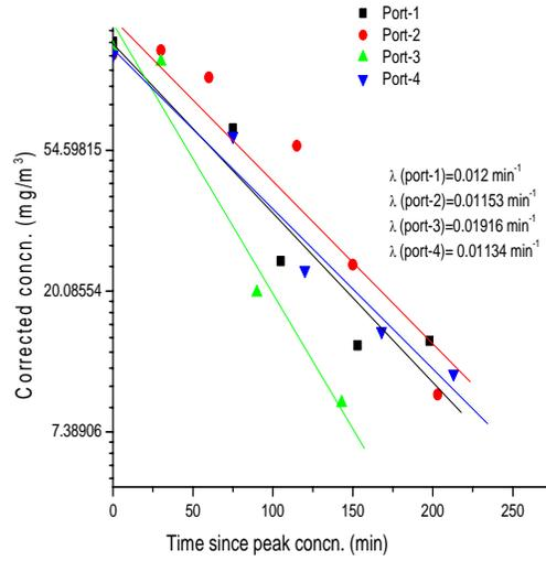
**Temporal variation of the corrected mass concentrations at the four sampling ports of CSF**
