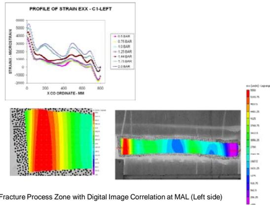
Fracture Process Zone with Digital Image Correlation at MAL (Left side)
