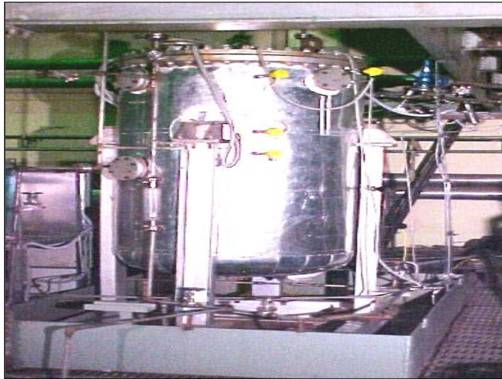
**Test Facility to study condensation in presence of non-condensable gas**
