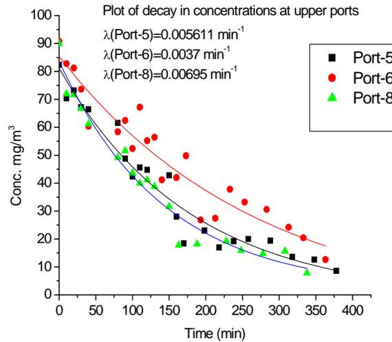
**Estimation of aerosol mass depletion constants from the exponential fit to the concentration vs. time plot at the lower and upper sampling ports**
