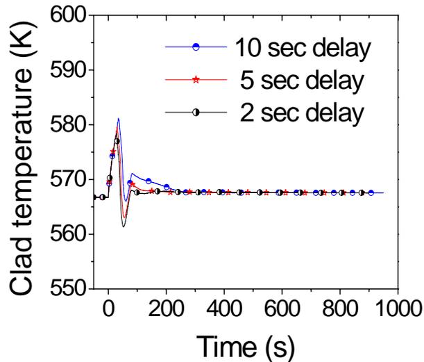
**Peak clad temperature profile during station black out and failure of both primary and secondary shutdown systems**
